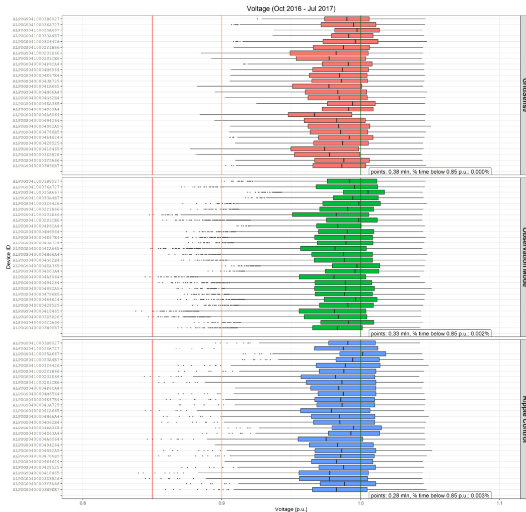
Figure 1. Voltage measurements (in p.u.) at grid connections over one year, from 01.10.16 to 30.09.17. The grid was operated in three different modes: activated GridSense, “observation mode” (periods without any grid level control) and “ripple control” (the previously used approach to control boilers and heat pumps). Over-voltage situations do not occur due to the modest prevalence of photovoltaic units in Riedholz. Voltage limits according to the European norm EN 50160 are indicated in orange and red (0.9 p.u., violation tolerable for a maximum of 5 % of time assessed on a weekly basis, 0.85 p.u., violation not tolerable). The figure is directly taken from SoloGrid’s final report [3].
